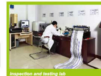
Inspection and testing lab For testing on parts or pens such as refill writing length, salt atmosphere test, constant temperature drier-cold & hot temperature cycling test, water boiling test, pull-out force test, hardness test, drop test stand
