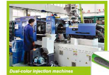
Dual-color injection machines For two-color plastic parts injection
