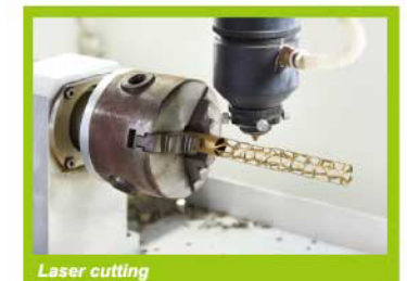
Laser cutting For permanent logo or artwork cutting on pen
