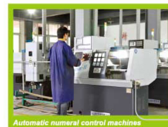
Automatic numeral control machines For metal parts such as tip, plunger, dome, mid-connector, band
